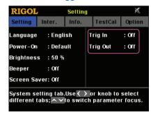
When multiple power supplies are in serial or parallel connection, enabling the external trigger function can realize the synchronous output for multiple power supplies.
